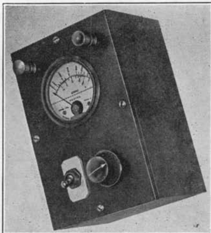
Figure 25. This ohmmeter is particularly useful for measuring resistances too low to be read accurately on an ohmmeter of the type illustrated in figures 21, 22 and 23.
