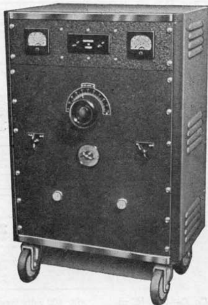
Figure 4. This de luxe 400-watt u.h.f. diathermy machine incorporates many safety features and worthwhile refinements. It uses two HF-200's in a push-pull Armstrong circuit.
