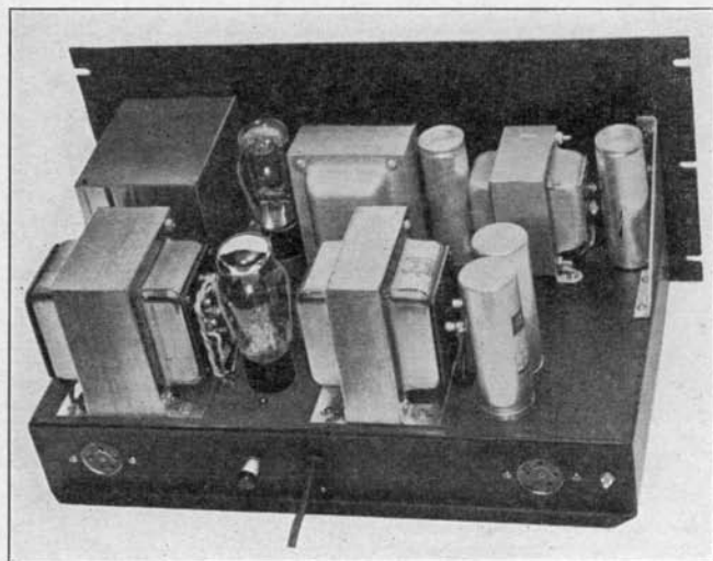
Figure 31. A dual power supply designed for supplying r.f. exciter and speech amplifier and driver stages. The smaller supply delivers 350 volts and is very well-filtered. The larger supply delivers 600 volts and is moderately well-filtered.
