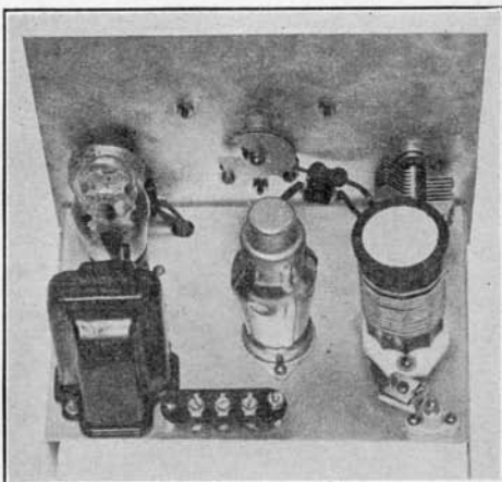
Figure 8. Showing arrangement of components in the standard "Gainer." The tube shield and short detector grid lead are necessary to avoid "grid hum."
